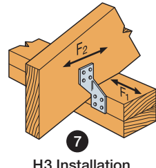
H3 Installation (nails into upper top plate)
