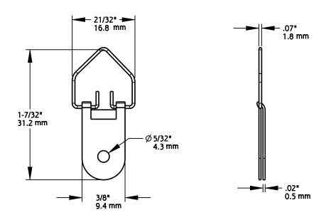
Material: Steel Finish: Zinc Plated Fasteners: Screw, #6x5/8"Pan(1 per)
