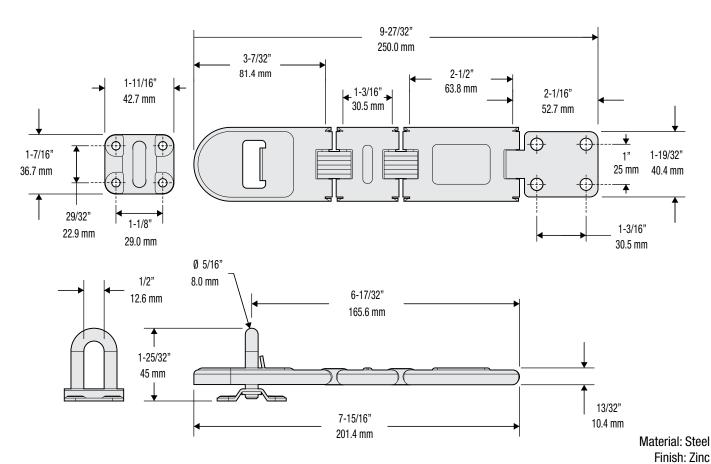
Fasteners: 8 Each #9 x 1" Flat Head Screws 2 Sets #10-32 x 2" Bolts with Nuts and Washers (not shown) Accepts up to 7/16" (11 mm) Padlock Shackle
