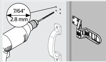
**C** Install and tighten screws.
