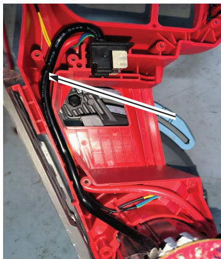
7) Press Black Wire into housing groove on top of the Red Wire.
